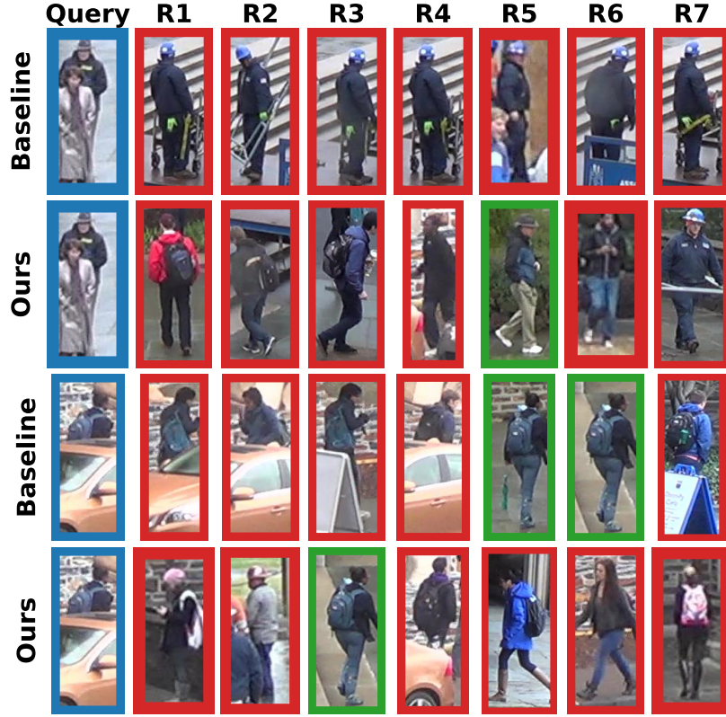
FIGURE 4 Visualization of retrieval results on hard samples. The leftmost column shows the severely occluded query images, followed by the top retrieved results from the gallery by the Baseline and our D 3 F framework. Green and red bounding boxes denote correct and incorrect matches, respectively. Benefiting from the injection of generative structural information, our method successfully infers the occluded topologies, demonstrating a distinct advantage over the baseline in retrieving challenging occluded targets.
