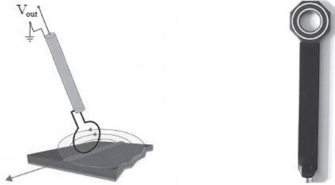
Figure 2.2 Working principle of the magnetic field probe and the structure of the electric field shielded magnetic field probe
