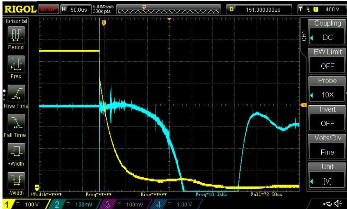
Fig. 3g. Experiment 242 ( B_4C+Al+LAH ) Yellow trace:- For ignition at medium-compression force, the applied voltage on the capacitor shows that after 140\mu s the rapid discharge is counteracted by a flow of charge from the plasma back into the capacitor over a period of 70\mu s . Turquoise trace:- Compression load measured during the ignition.
