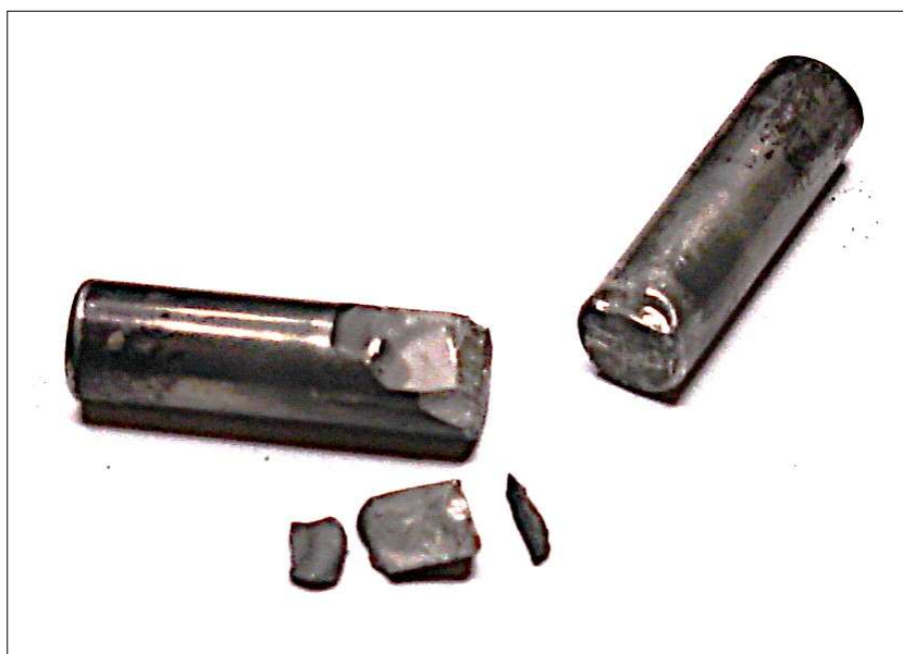
Fig. 2c Experiment 223 ( \text{ZrN}+\text{Zn}+\text{LAH} ) An anvil shattered due to the small wedge shown. The opposing anvil shows damage on the contact face.
