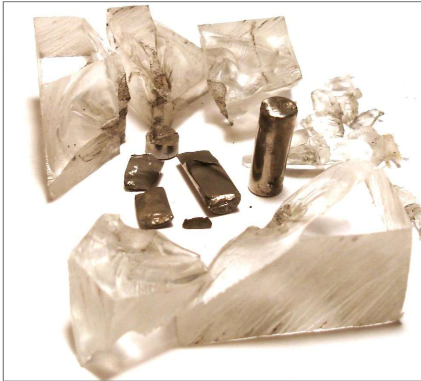
Fig. 2d Experiment 249 (WC+LAH) One anvil shattered due to the shock wave started by the small wedge shown. The opposing anvil shows damage on the contact face. The acrylic cell was shattered by the shock-wave.
