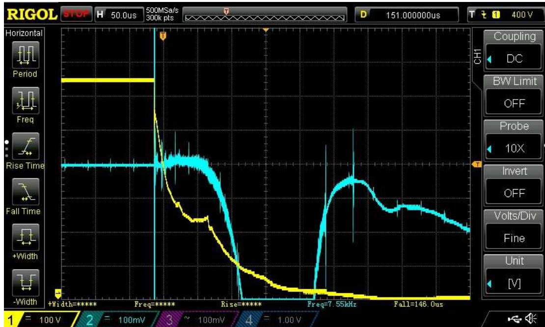
Fig. 3e. Experiment 234 (SiC+Zn+LAH) Yellow trace:- For ignition at medium-compression force, the applied voltage on the capacitor shows that after 50\mu\text{s} the rapid discharge is counteracted by a flow of charge from the plasma back into the capacitor over a period of 50\mu\text{s} . Turquoise trace:- Compression load measured during the ignition.
