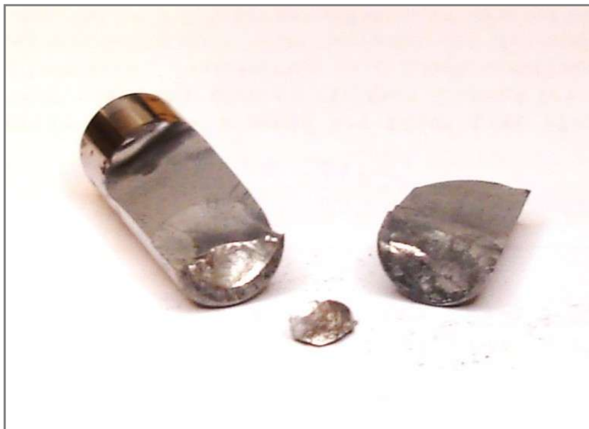
Fig. 2b Experiment 225 ( \text{ZrC}+\text{Zn}+\text{LAH} ) An anvil shattered due to the small wedge shown. The opposing anvil was pitted but not broken.
