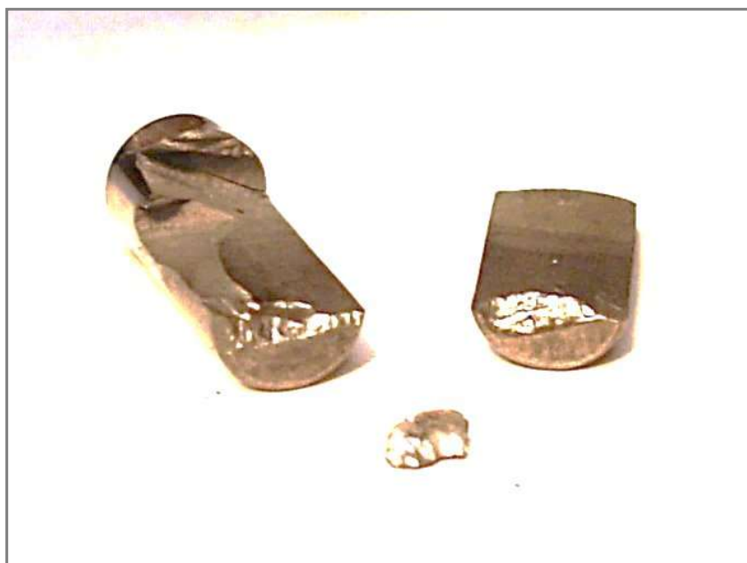
Fig. 2a Experiment 228 ( B_4C+Zn+LAH ) An anvil shattered due to the small wedge shown which was formed under extreme pressure. The opposing anvil (not shown) was pitted but not broken.
