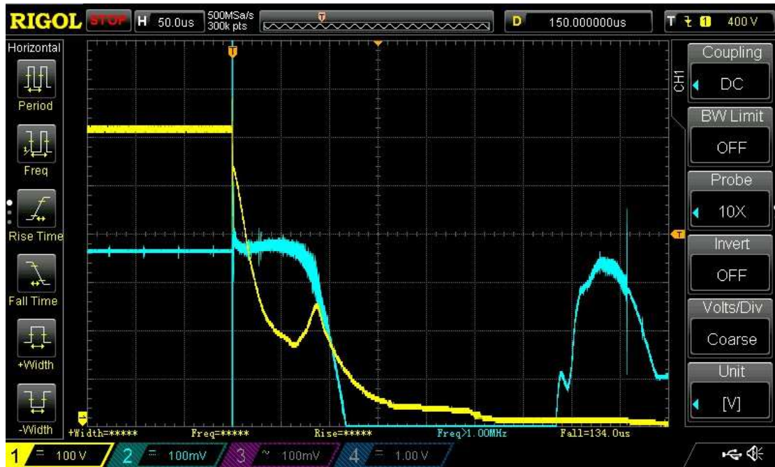
Fig. 3d. Experiment 230 (WC+Zn+LAH) Yellow trace:- For ignition at medium-compression force, the applied voltage on the capacitor shows that after 70\mu\text{s} the discharge is counteracted by a flow of charge from the plasma back into the capacitor over a period of 50\mu\text{s} . Turquoise trace:- Compression load measured during the ignition.
