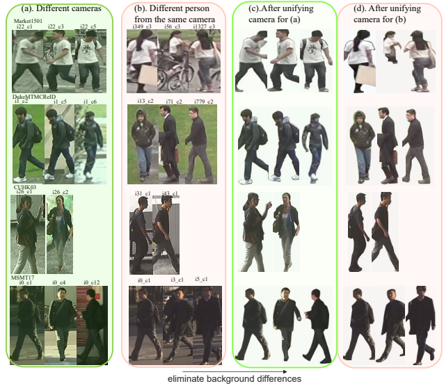
Figure 1. a. Reflect the background variations introduced by different cameras. b. Highlight the strong semantic consistency of images of the same pedestrian captured by the same camera. c & d. Demonstrate how we align images to approximate a Gaussian white-noise background by eliminating camera-specific variations.
