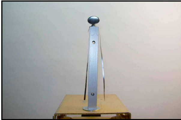
Fig. 1: Uncharged electrostatic demonstrator
