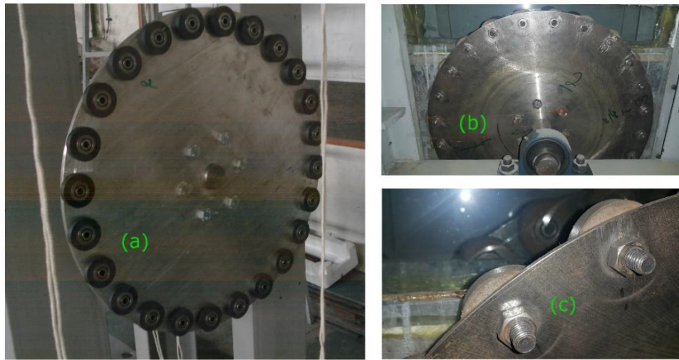
Fig. 4. a) Display of one of the two disks in the experiment illustrating the arrangement of 24 magnetics in a circular manner, b) the same with the magnetics facing away and showing the back of the disk, c) and a close-up of the several magnets facing one another in the actual configuration used in these experiments with the two disks.
