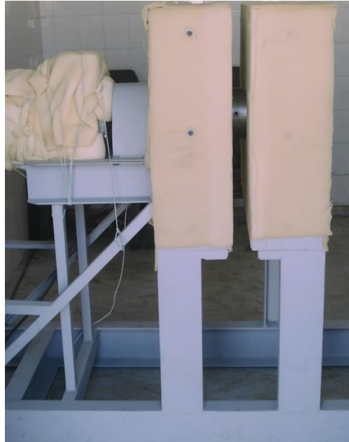
Fig. 5. Illustration of the foam system used to cover the metal boxes surrounding the rotatory disks in the experiments, the purpose of which was to avoid the effects of any errors as caused by the movement of air from the rotation of disks and internal vibrations of the system.
