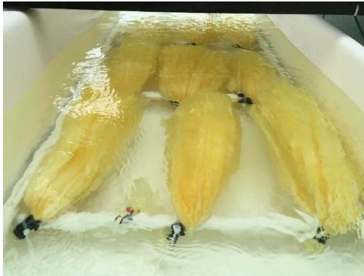
"Material designed to capture uranium from seawater as an alternative to land-based mining of the fuel for nuclear power production is tested at PNNL's Marine Sciences Laboratory. Credit: PNNL"
