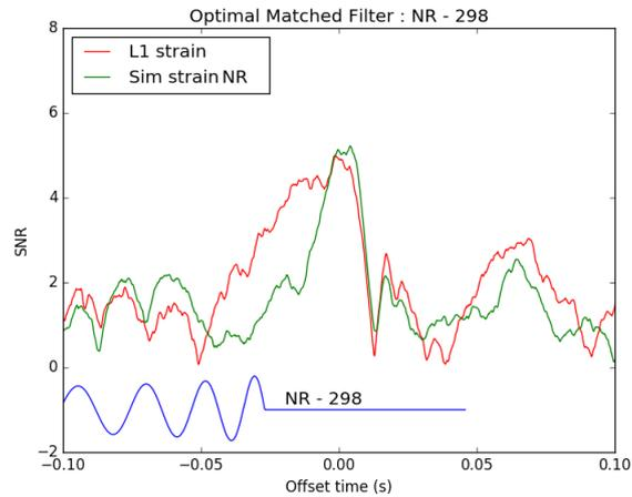
**Fig 14:** Optimal matched filtering results using the NR-298 signal (in blue) as a template, applied to process real data and simulated data (obtained by adding the NR signal to the recorded noise in Livingston). The red curve is the result of filtering the real data and the green curve is the result of filtering the simulated data.
