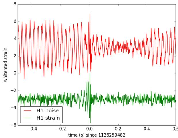
**Fig 18:** Curves obtained processing the real data (H1 strain) with the standard whitening filter (in green) and the UWF-NBP (in red), from 31.5 to 43.5Hz
