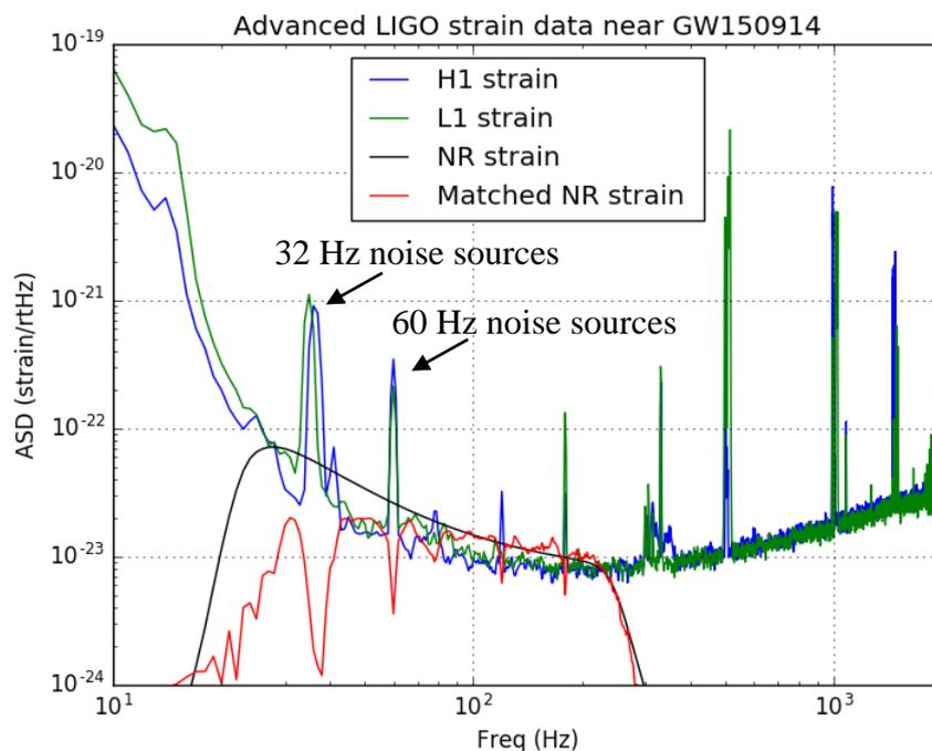
**Fig 6:** Frequency power spectrum of signals from LIGO's GW150914 event.
