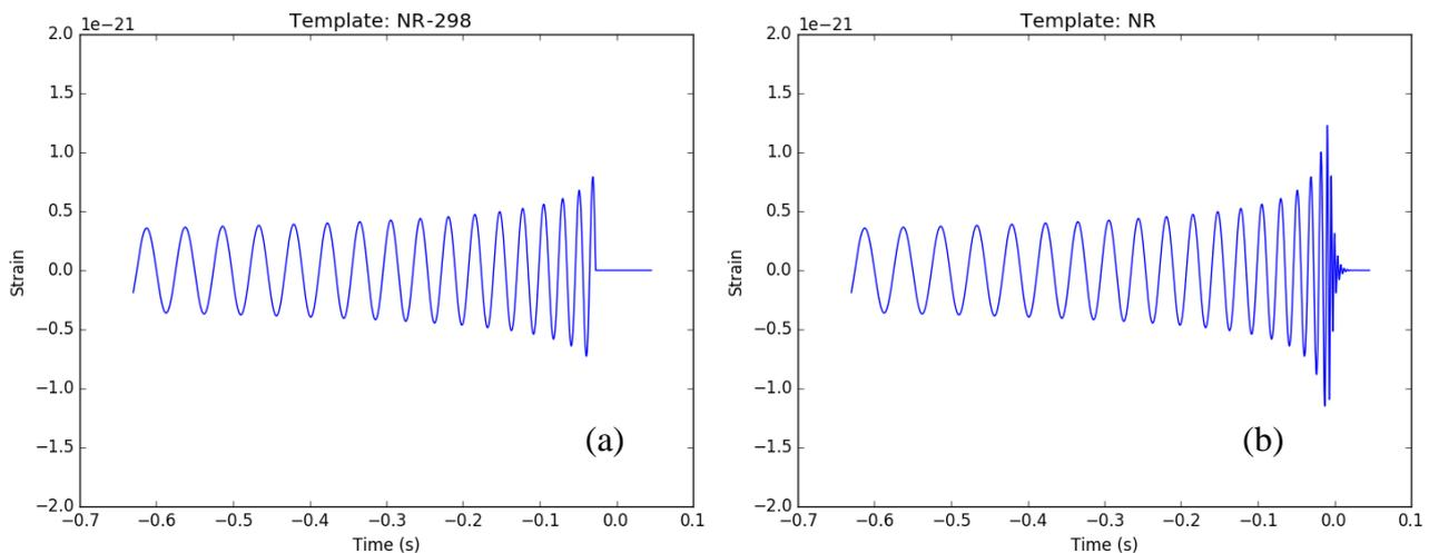
**Fig 13:** Two waveform templates: a) NR-298 - NR signal with the final 0.0727s (final 298 curve points) set to zero; b) Original NR signal.
