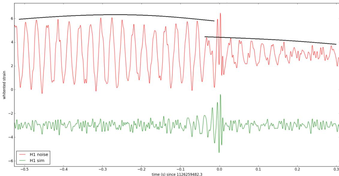
**Fig 20:** Same curves from Figure 15 in a larger scale. The red signal is basically a 32 Hz noise and the two black lines represent the level of this noise after and before the time of the GW150914 event
