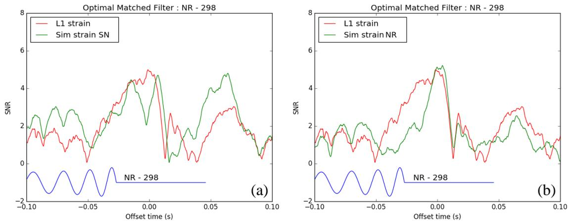
**Fig 16:** Optimal matched filtering (using the NR-298 signal in blue as a template) results: a) Processing the real data (L1 strain, in red) and the simulated data (in green) obtained by adding the SN signal to the noise recorded in Livingston; b) Processing the real data (L1 strain, in red) and the simulated data (in green) obtained by adding the NR signal to the noise recorded in Livingston
