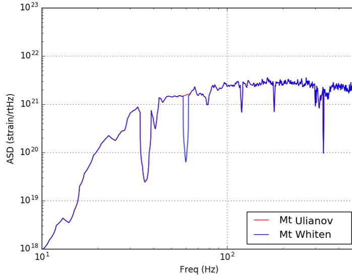
**Fig 21:** Gain curves used in the whitening filter (in blue) and the UWF-NBP, from 57.5 to 63.5 Hz (in red)
