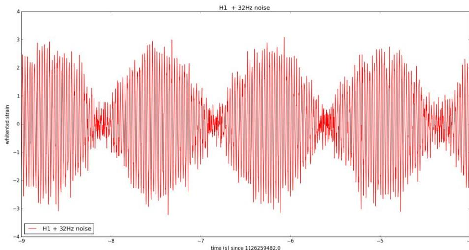
**Fig 24:** 32 Hz Noise of detector in Hanford modulated by a lower frequency signal in the range of 2.5 Hz
