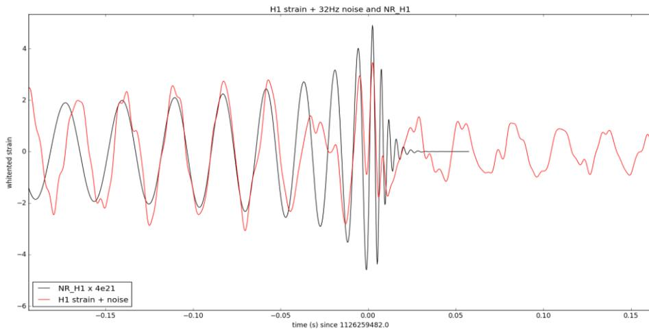
**Fig 19:** Curve of the NR signal (multiplied by  $4 \times 10^{21}$ ) and 32 Hz noise signal, obtained by processing the real data with the UWF-NBP, from 31.5 to 43.5Hz
