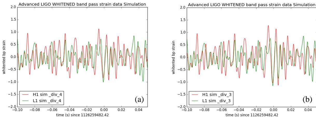
**Fig 11:** Results of the whitening filter process: a) Simulation using the NR signal divided by 4; b) Simulation using the NR signal divided by 3.
