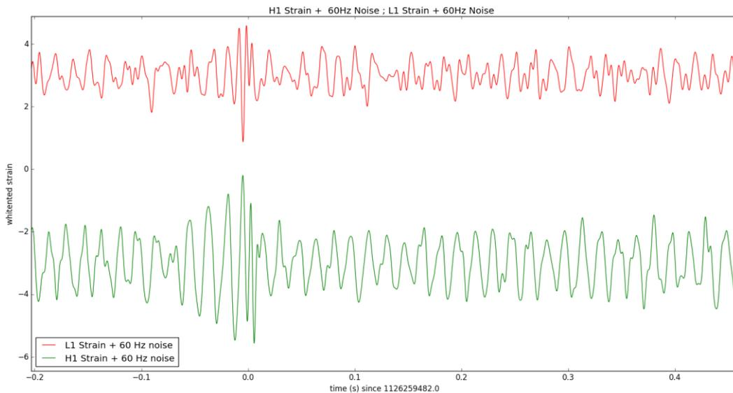
**Fig 22:** Curves obtained by processing the real data with the UWF-NBP (from 57.5 to 63.5 Hz), resulting in a 60Hz noise added to the L1 and H1 strain signals
