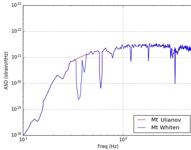
**Fig 17:** Gain curves used in the “standard” whitening filter (in blue) and in the UWF-NBP (in red), from a range of 31.5 to 43.5Hz
