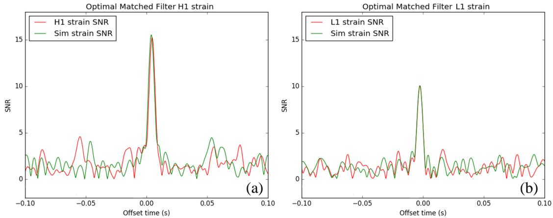
**Fig 12:** Results of optimal matched filtering. a) Hanford (H1) detector: real data (in red) and simulated signal (in green); b) Livingston (L1): real data (in red) and simulated signal (in green).
