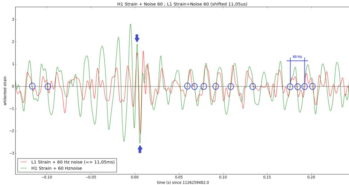
**Fig 23:** Same curves from Figure 19 with the L1 strain curve (not inverted) shifted to 11,05ms. The blue circles represent some points where the 60Hz noise signals have the same phase.
