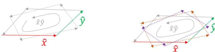
Fig. A1.2 The same bivector all the time. Rotating its vectors, does not change the bivector (it is always the same as long as it represents the same plane -magnitude and orientation left aside-).
