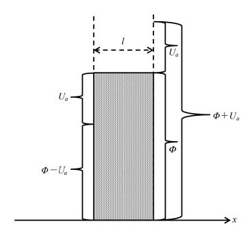
Figure 1: Variation in height of barrier in both sides due to applied voltage
