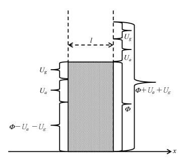
Figure 2: Variation of the heights of potential barrier in both sides of due to applied voltage  $U_a$  and density gradient.  $U_g$  is the variation in potential due to the density gradient.
