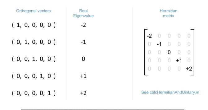
As an example, here are the position state vectors. Each one corresponds to a position value. Mathematically, a basis of orthogonal vectors and a corresponding set of real eigenvalues are the parameters needed to specify a Hermitian matrix. In other words, if you have these you can compute a Hermitian matrix, and also vice-versa. If you're interested in the details, check out *calcHermitianAndUnitary.m* in the companion code.
