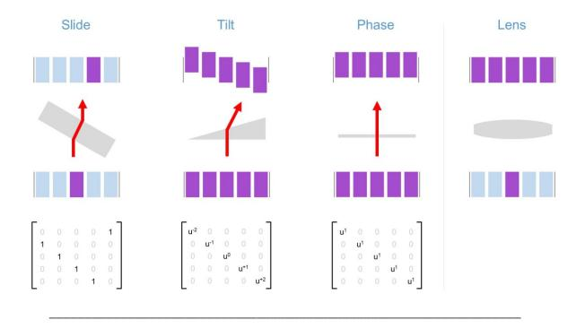
These are the 3 basic transformations slide, tilt and phase, and each one corresponds to an optical device. But more precisely, these transformations describe *ideal* devices. In practice, actual devices behave differently, and the picture becomes more complex.
