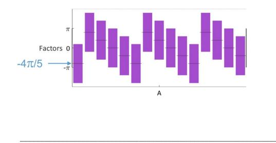
Let's see an example. Here's an angle state. The phase goes through 3 cycles, so the angle is +3. The slide transformation shifts every component to the next position.
