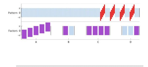
To analyze the grating, we simply extrapolate further to more factors. A grating is composed of an angle factor A, a position factor B, angle factor C, and position factor D.
