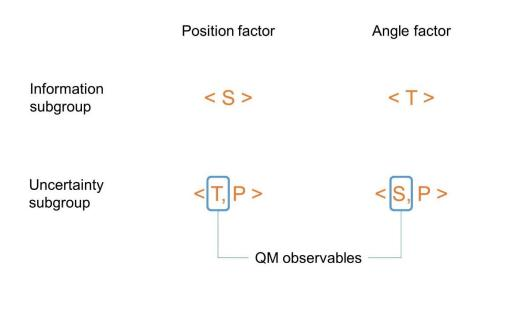
This chart summarizes our analysis of optical factors. For a position factor, slide generates the information subgroup, while tilt and phase generate the uncertainty subgroup. For an angle factor, tilt generates the information subgroup, while slide and phase generate the uncertainty subgroup.
