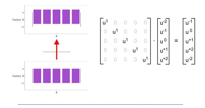
The final basic transformation is the *phase* transformation. Phase is physically implemented by an optical window. This is a thin piece of glass with both faces perpendicular to the optical axis. The glass has a higher index of refraction than the air or vacuum around it, and so the window shifts the phase by some amount, compared to the case with no window.
