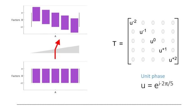
We have been discussing the slide transformation. Now we'll move on to the *tilt* transformation. Tilt is physically implemented by an optical wedge. This is a piece of glass with two faces. The first face is perpendicular to the optical axis, the second face is at some angle to it. In terms of geometric optics, a ray passes through the first face without changing angle. But at the second face, the ray is refracted and it continues on, propagating off into space at some new angle.
