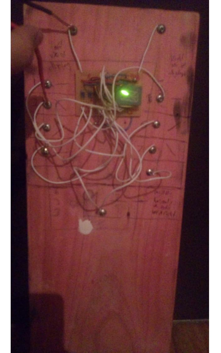
Testing screw 3 (negative on ground, positive on screw 3):
