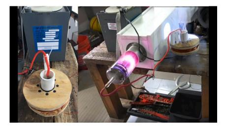
For a 1 g of Al foil probe, a horn antenna of 20 W was used; the power at the probe was about 1 W.
