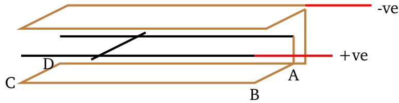
FIGURE 3. Tripled Railgun Design. Main rails black; loop current rails brown.
