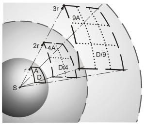
1. SPHERE'S SURFACE AREA & DENSITY INTENSITY OR DENSITY OF AN EXPANDING SPHERE'S SURFACE AREA, D \alpha (IS PROPORTIONAL TO) 1/r2
