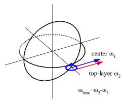
Fig.9 One convective ring at the equator, the speed difference causes a beat frequency.
