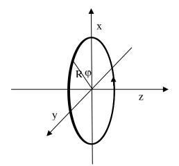
Figure 1: One-dimensional circular current loop
