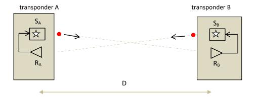
Initially  $S_A$  emits a short light pulse, which is detected by  $R_B$ , which triggers  $S_B$ , which immediately emits a short light pulse, which is detected by  $R_A$ , which triggers  $S_A$ , which immediately emits a short light pulse, which is detected by  $R_B$ , and so on.
