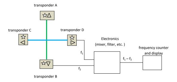
The rod of transponders A and B (rod AB) could be pointed towards Leo, whereas the rod CD is rotated to be parallel or perpendicular to rod AB and the frequency change noted. It is important that the pulse counting be made over relatively long time interval for better accuracy and to average out spurious signals.
