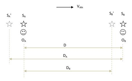
$S_A$ ' is the apparent position of  $S_A$  as seen by  $O_B$ , and  $S_B$ ' is the apparent position of  $S_B$  as seen by  $O_A$ , where  $O_A$  and  $O_B$  are the detectors at A and B, respectively.
