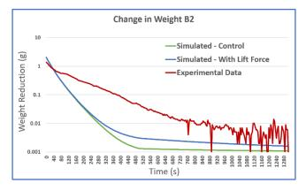
Figure 4: Experimental data showing reduction in measured mass.
