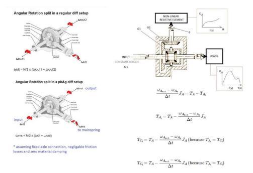
2. Describing the road as linear gradients and following a change in gradient to resistance on and absorbed by the mainspring component. I have made a small start on looking at the relevant equations:
