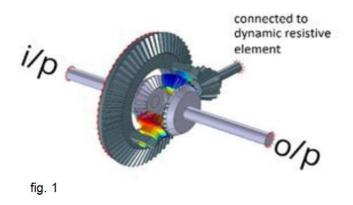
I realised quickly that the resistance on the output axle would only cause the ring gear to spin, so I questioned what would give the ideal resistance to act on the ring gear. I decided that a ratcheted spring (aka a pull-back motor) would be an intuitive choice as a resistive element on the differential's ring gear to stop it spinning freely.
