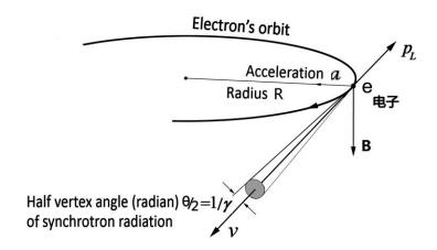
Figure 2. Radiation angular distribution of moving electrons
