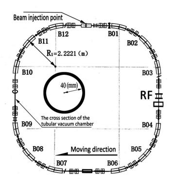
Figure 1. Layout diagram of HLS800MeV electronic storage ring
