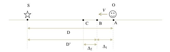
With the same argument as before, during the time interval that light moves from the source to point B, the observer moves from point A to point B.
