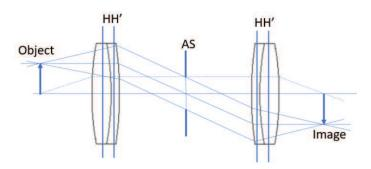
Fig.3 Double telecentric optical relay
