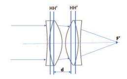
Fig. 1 Two cemented doublets lens group
