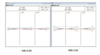
Fig.4 Cemented doublets wave aberrations graphs
