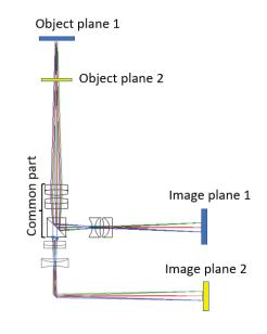
Fig. 4 Apparatus for imaging an object in multichannel position
