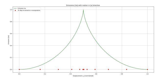
Figure 4: Emissions in [a] as a function of displacement in the same direction. Displacement has been normalised by dividing by  $P_a = \tau \pi$ . Red dots indicate sample locations of the reactive end, and show how it initially moves quickly, slows to a momentary stop, and then quickens its displacement again.
