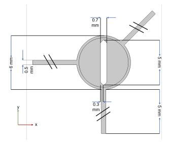
Fig. 1. Shows the micromixer environment and all the relevant dimensions. In the center of mixing chamber, a microrobot is placed with a sharp edge to improve mixing efficiency.
