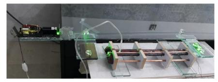
Fig. 9. Experimental apparatus setup with horizontal electrical magnet
