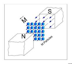
Fig. 15. The M Domain Direction as denoted by ( M )
