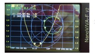
Figure 3: Display of the VNA. At resonance (2401 MHz), the SWR is less than 1.3 (yellow U-curve). The green circle shows how much the reactance changes as a function of frequency.
