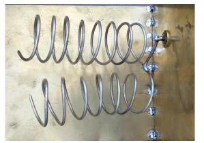
Figure 2: Double helix in front of the 90° reflector. On the right you can see the backside of the coax socket. The 20 mm short piece of wire to the helix simplifies the electrical matching (see text). For continuous operation a mechanical fixation of the helix is recommended to avoid a short circuit with the reflector.
