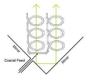
Figure 1: The angle mirror deflects every wave coming from above by exactly 180°. This also applies to waves arriving at an angle. Only on the short horizontal path below the helix the polarization sense is inverted.
