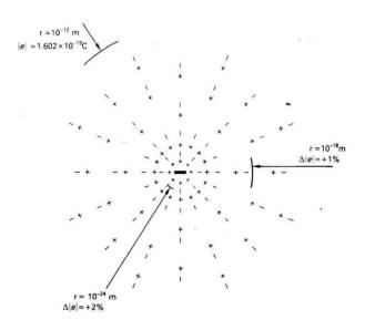
Fig.1 : The electron is screened by virtual pairs  $(e^-, e^+)$  in the concept of vacuum polarization of QED. This figure is scanned from Fig. 13.1 in the textbook "Nuclear and Particle Physics " by W.S.C. William
