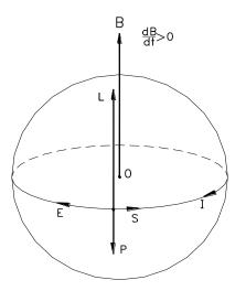
Fig. 10 : Direction of spin S of the electron in the time-varying **B** when  $d\mathbf{B}/dt > 0$ . The electron spins up :  $\mathbf{L} \uparrow \uparrow \mathbf{B}$ .
