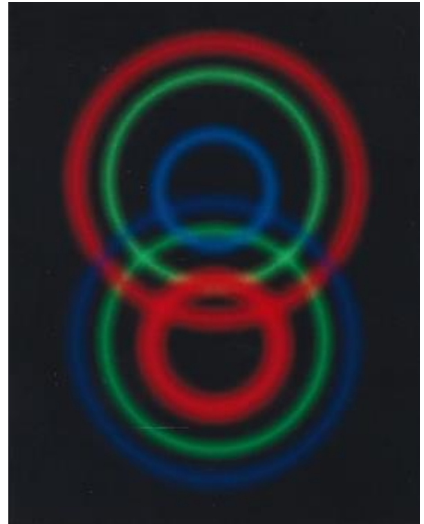
Figure 1: Conservation of energy by PDC. Anton Zeilinger [11] and Y.S. Lee [12] have shown that the ultra-violet laser incidence on a non-linear crystal through the process of PDC to lower energy photons. Thus, allows each photon to be split into two of longer wavelengths. The individual photon energy became an inversely proportion of their initial wavelength, increasing the associated quantum expansion by a 16 times decreasing density and increasing the associated space volume.
