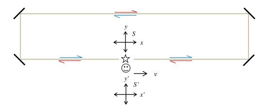
The light source and the observer are co-moving to the right with velocity v. Consider two inertial frames S and S'. S is the lab frame. S' is the reference frame of the observer. S' is moving with velocity v in the +x direction relative to S. The observer and the source are both at the origin of S'.
