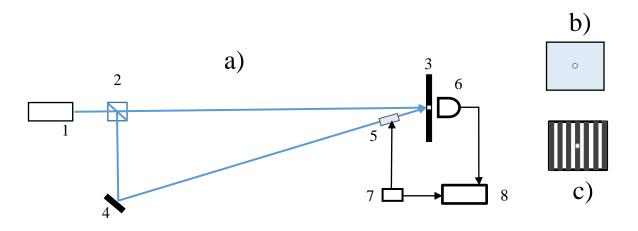
Figure 1. a) The basic scheme of the proposed installation. 1 - laser, 2 - beam splitter, 3 - screen with a pinhole, 4 - mirror, 5 - optical shutter, 6 - detector, 7 - shutter control source, 8 - registration system. b) View of the illuminated screen with a single beam. c) View of the illuminated screen with two beams.
