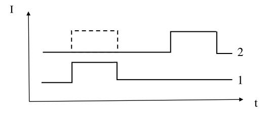
**Figure 2.** The expected results of the experiment. 1 - oscillogram of the voltage applied to the optical shutter. 2 - radiation intensity recorded by the detector.
