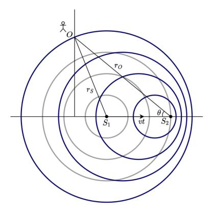
Figure 5: Doppler shift for a moving source
