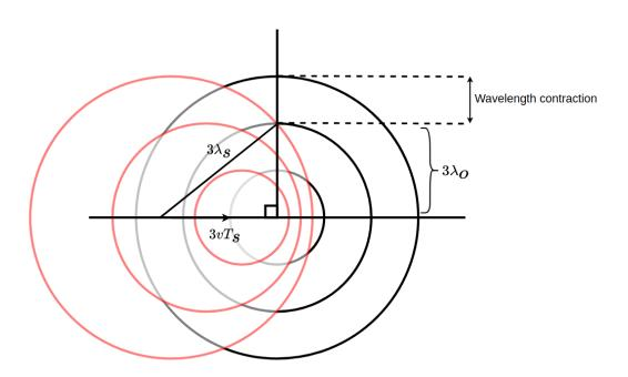
Figure 3: Transverse Doppler shift for a moving source
