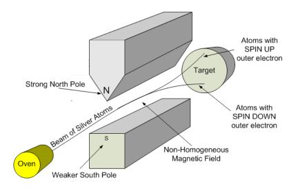
However if the electron was actually physically spinning then the result of the Stern-Gerlach experiment could be explained as follows -
