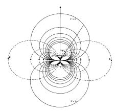
Figure 1: Equipotential (V, solid lines) and electric field (E, dashed lines) in a dipole field <sup>2</sup>
