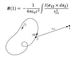
Figure 1: The magnetic field from a current is obtained from an integral around the circuit
