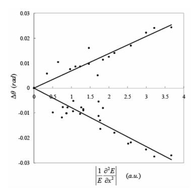
Fig. 5. Correlation between the second derivative of the electric field and the angle change  $\Delta\theta$  (the data of  $|\Delta\theta| > 0.005$ rad is displayed).
