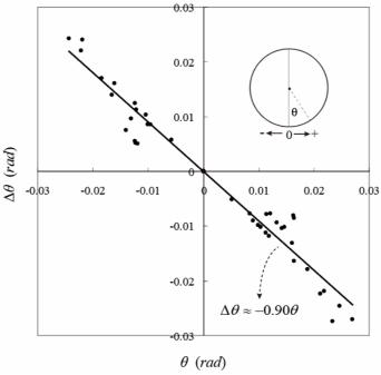
Fig. 4. Correlation between the moving direction  $\theta$  of the photon and the angle change  $\Delta\theta$  (only  $|\Delta\theta| > 0.005$ rad is displayed).
