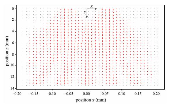
Fig. 2. Two-dimensional map of photon movement. When multiple vectors are measured, only the vector of maximum intensity is displayed. The length of the vector is normalized with data in each row.
