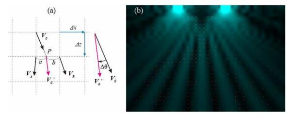
Fig. 3. Angle change of photon motion. (a) Method of calculating angle change  $\Delta\theta$  using measured vectors  $V_0$ ,  $V_A$ , and  $V_B$  ( $\Delta x$  and  $\Delta z$  are measurement intervals). (b) Two-dimensional distribution of  $\Delta\theta$  (indicated by red dots).
