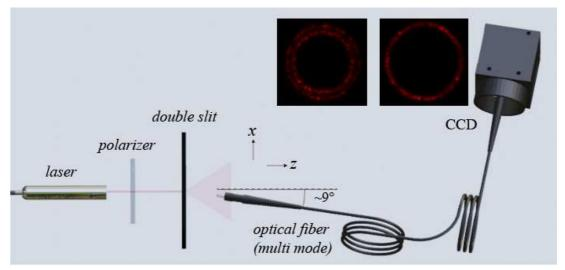
Fig. 1. Apparatus for observing photon motion using fiber. Laser beam (635nm) passes through a polarizing plate (45°) and a double-slit (slit width =  $20\mu m$ , interval =  $100\mu m$ ) to form interference fringes. The interference light enters the optical fiber (inclination is 9°, diameter =  $50\mu m$ ) and is detected by the CCD placed at the tip. A motorized stage scans the optical fiber in the x and z directions to obtain a distribution of photon movement.
