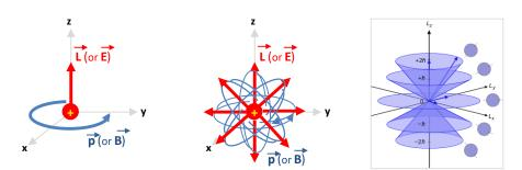
Figure 7a (left). Illustration of using  $\vec{L}$  vector to represent  $\vec{E}$  vector, and using the particle's trajectory (or the  $\vec{p}$  vector) to represent  $\vec{B}$  vector.
