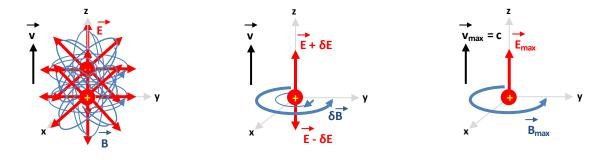
Figure 3a (left). When a positive point-charge starts to move in +z direction, its  $\vec{\mathbf{E}}$  (or  $\vec{\mathbf{B}}$ ) partially overlapped one on another. Figure 3b (middle). The net effect of Figure 3a on the z axis (when  $|\vec{\mathbf{v}}| > 0$ ). Figure 3c (right). The net effect of Figure 3a on the z axis (when  $|\vec{\mathbf{v}}| = c$ ).
