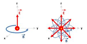
Figure 1a. Assumption: a static positive point-charge having its one electric field  $\vec{E}$  line pointing to the +z direction will produce a circular (closed) magnetic field  $\vec{B}$  line in x-y plane.
