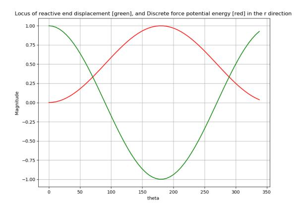
Figure 5: The locus of motion of the reactive end follows a  $cos(\theta)$  dependency for each axis, whereas the potential energy follows  $sin^2(\theta/2)$ .
