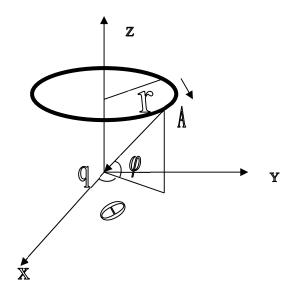
As shown in the figure: the solenoid with radius R is arranged along the z-axis, and the charge q moves at the speed  $V_2$  along the x-axis at the origin. We need to calculate the force of the solenoid on the charge q.
