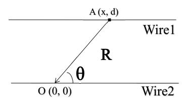
As shown in the figure above, there are two infinitely long parallel wires with a distance of  $\mathbf{d}$ . We want to calculate the stress condition in wire 2.
