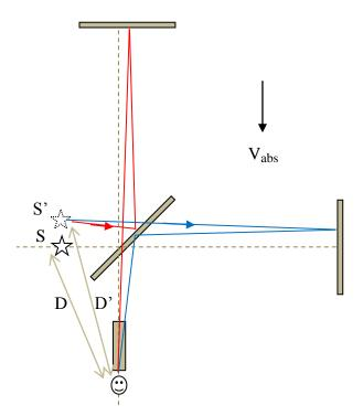
The path lengths of the longitudinal (blue) and the transverse (red) light beams are changed slightly *differently* due to absolute motion, and hence causing a small fringe shift.
