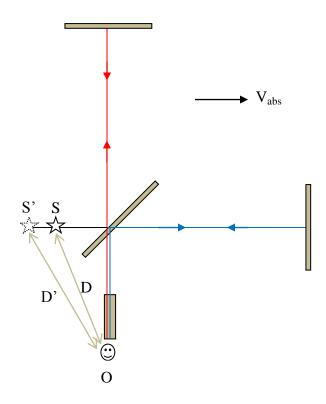
As we can see from the above diagram, absolute motion of the Michelson-Morley interferometer causes only an apparent change in the point of light emission relative to the observer, from S to S'. The velocity of light is always constant c relative to the observer, regardless of the absolute velocity of the interferometer.
