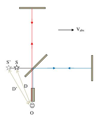
As we can see from the above diagram, absolute motion of the Michelson-Morley interferometer causes only an apparent change in the point of light emission relative to the observer, from S to
