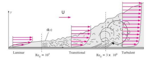
Figure 1. Incompressible Flow over a Flat Plate - not to scale.
