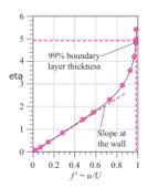
The Blasius profile in similarity variables for the boundary layer growing on a semi-infinite flat plate. Experimental data (circles) are at  $Re_x = 3.64 * 10^5$ .
