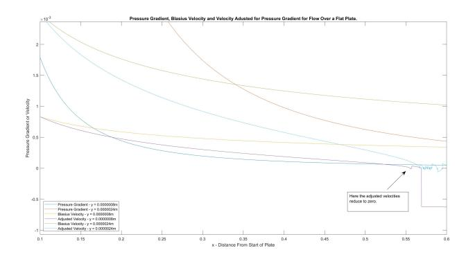
Figure 6. Pressure Gradient and Adjusted Horizontal Velocity
