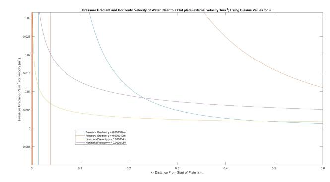
Figure 4. Calculated Pressure Gradient and Horizontal Velocity
