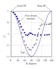
Pressure coefficient as a function of angle b along the surface of a circular cylinder; the solid blue curve is the irrotational flow approximation, blue circles are from experimental data at Re  $-2*10^5$  – laminar boundary layer separation, and gray circles are from typical experimental data at Re  $-7*10^5$  – turbulent boundary layer separation.
