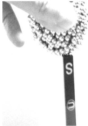
Figure 1: Sphere of ball magnets attracts the S pole of a bar magnet.
