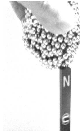
Figure 2: Sphere of ball magnets attracts the N pole of a bar magnet.
