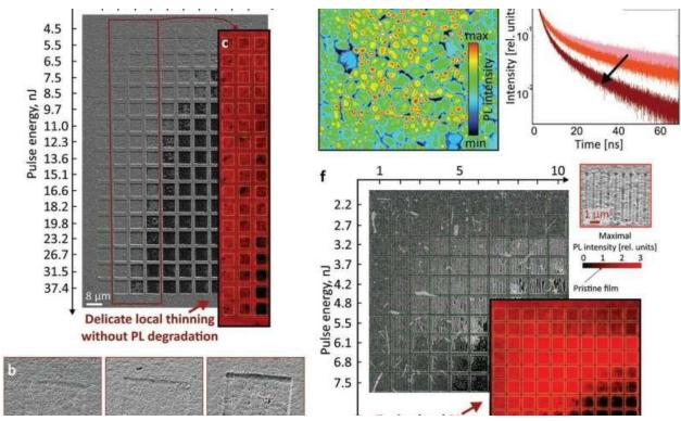
Tailoring local PL properties via precise laser-induced thinning and nanopatterning of MAPbI3 films. a)
