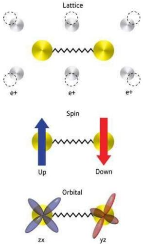
Shimojima and colleagues were surprised to discover that interactions between electron spins do not cause the electrons to form Cooper pairs in the pnictides. Instead, the coupling is mediated by the electron clouds surrounding the atomic cores. Some of these so-called orbitals have the same energy, which causes interactions and electron fluctuations that are sufficiently strong to mediate superconductivity.
