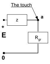
Fig. 1: Our equivalent scheme. "Z" is our "Rint". The generator is thus {E,Z}. E here is 220V. Point a denotes the metal body of the generator, which can be touched by the student, and where, in the case of the fault, a dangerous voltage arises.
