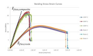
Figure 3. Bending results for the materials.
