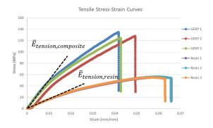
Figure 2. Tensile results for the materials.
