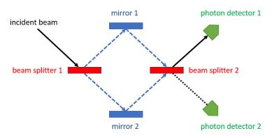
Figure 14: The Mach-Zehnder interferometer
