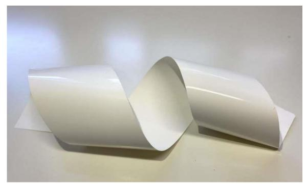
The team say that the mechanical robustness and operability of the flexible composite sheet at a wide range of temperatures makes it a promising electrolyte for Li-metal batteries. Credit: Tokyo Metropolitan University
