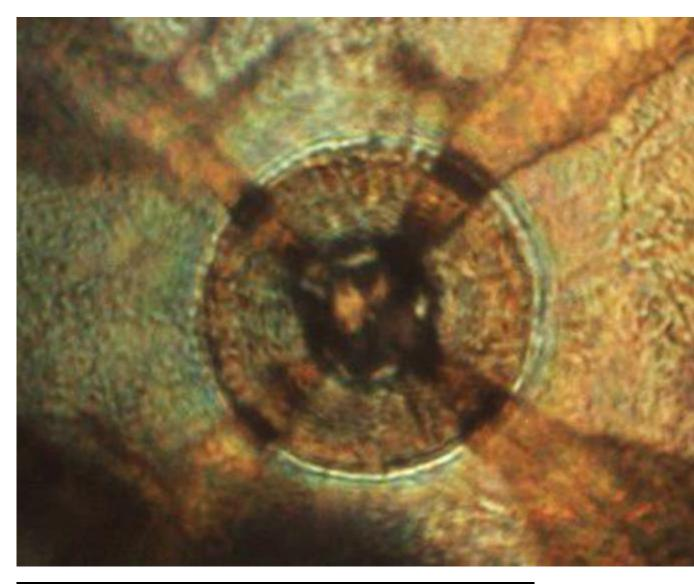
**TAKE THE PRESSURE** When crushed between two diamonds and cooled, a purported superconductor (shown here in a view through the diamonds) appears.
